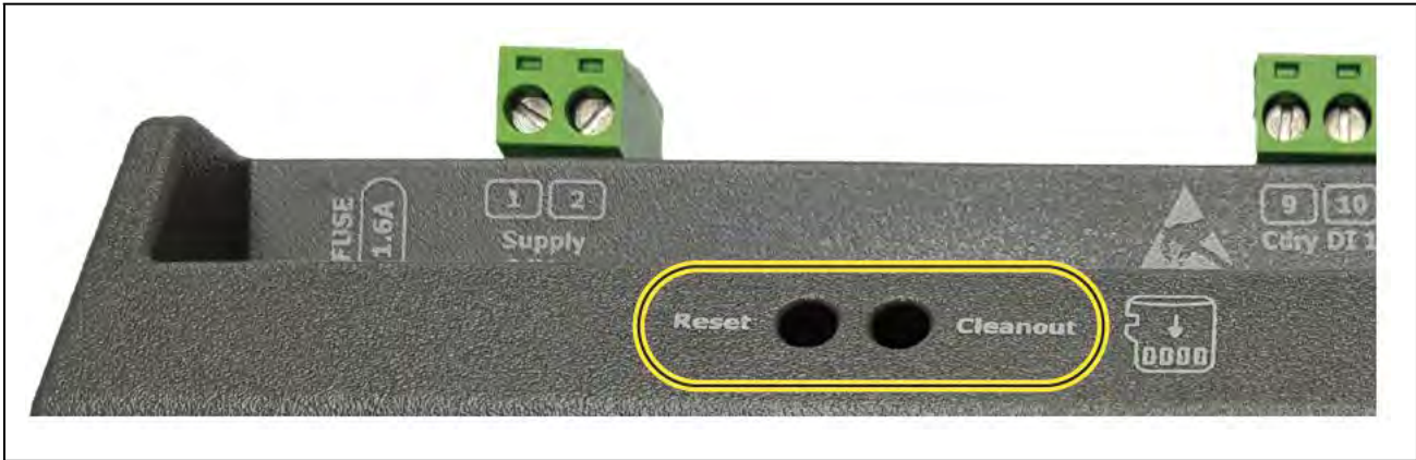
Site Supervisor Reset and Cleanout
