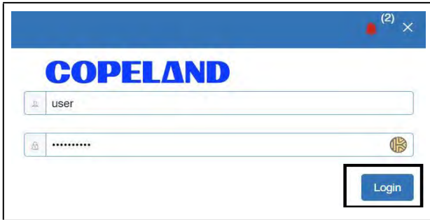
Figure 4-23 - Logging In to the Supervisory Controller
