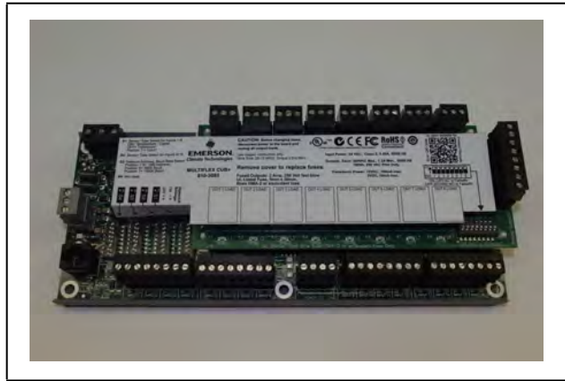
Figure 7-6 - MultiFlex Condensing Unit (CUB)
