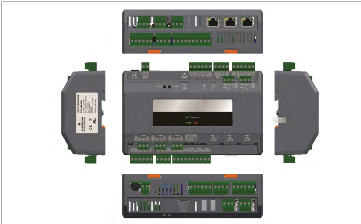
Figure 3-4 - Site Supervisor Detail
