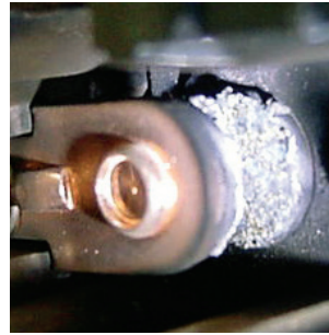
TRADITIONAL CONTACTORS after 300k cycles
